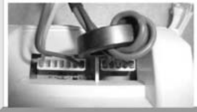
Picture F11-1: Open circuit/short circuit control between the motor phase cables covered with nucleus
